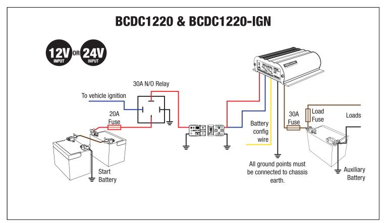
Figure 2.7d - Standard setup for a 24V Start Battery using relay for ignition switch
