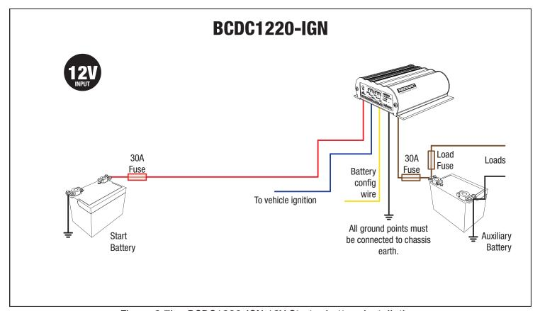
Figure 2.7b - BCDC1220-IGN 12V Starter battery installation
