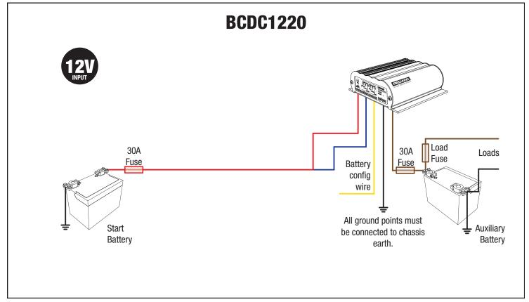
Figure 2.7a - BCDC1220 12V Starter battery installation
