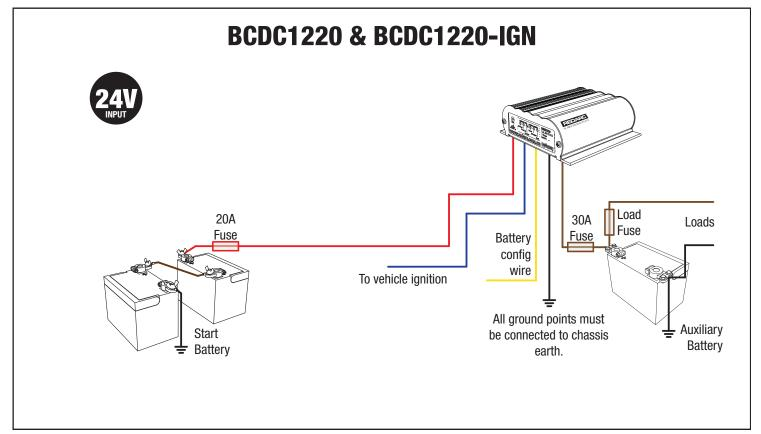
Figure 2.7c - BCDC1220 & BCDC1220-IGN 24V installation
