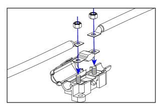
REDARC offer MIDI fuse kits containing the required fuses, fuse holders, crimps and nuts:
